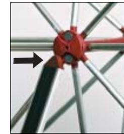
2/ When mounting the quick fit **magnetic bars**, just attach the top edge of the bar to the "hub" and the bottom edge will position itself automatically.
